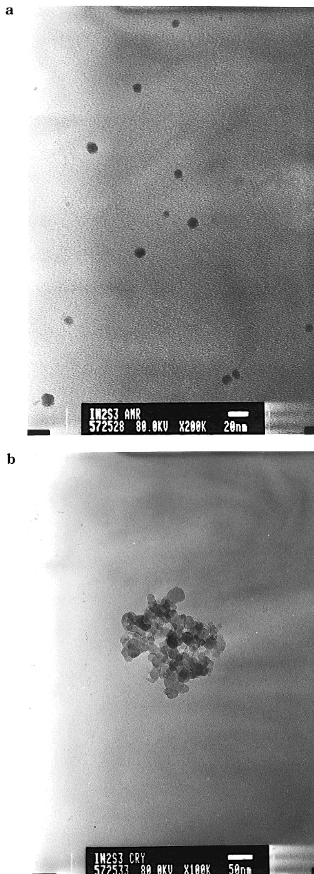
Figure 4. (a) TEM image of the material prepared at 0 °C. Scale: 0.5 cm = 20 nm. (b) TEM image of the material prepared at room temperature. Scale: 0.6 cm = 50 nm.
